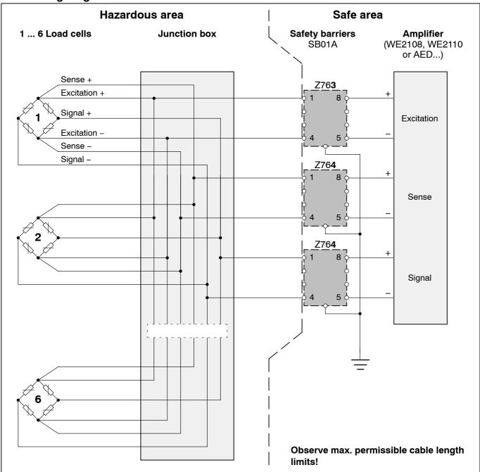
In accordance to the values of inductivity and capacity specified in the certificate of conformity, the following cable length limits between the safety barriers and the junction box are permissible with HBM cable type KAB8/00-2/2/2 (blue):
